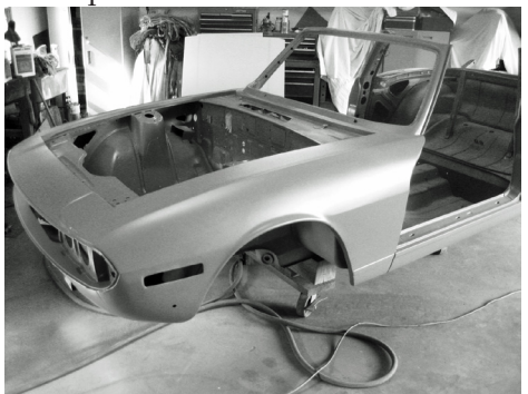
#3016 Seal coat applied
