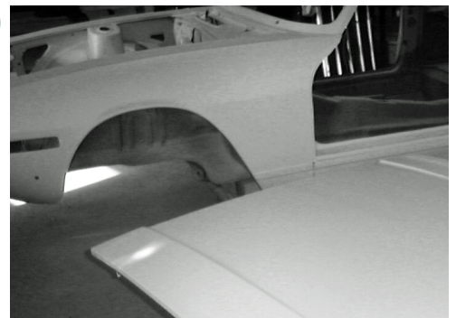
#141 Primer surfacer applied to bonnet
