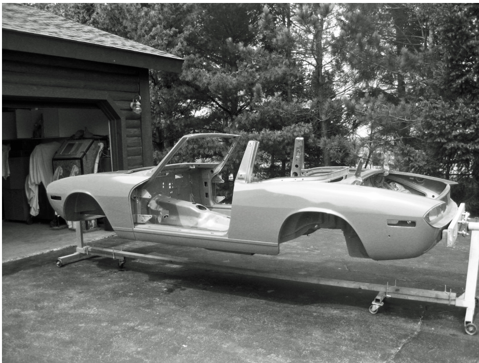
#0096 After 6 coats of top coat paint
