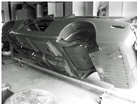
#3013 Epoxy bare metal applied to body tub
