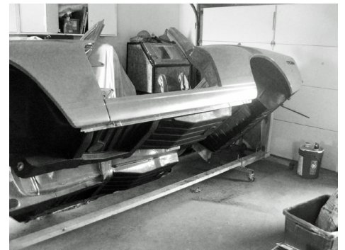
#109 Body "Schutz" undercoating applied
